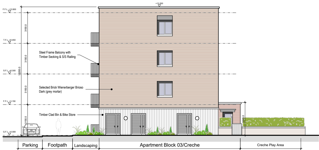
Apartment Block 03 - South Elevation Scale 1:200
